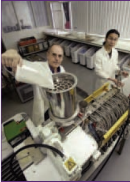
Paul Ainsworth and Sing Kwei manufacturing extruded foods prior to measuring their composition using microwave technology.
